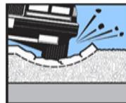
4. When vehicles drive over this cavity, the pavement surface cracks and falls into the hollow space leading to the birth of another pothole.
